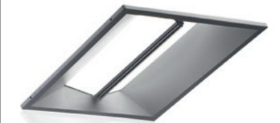
POWER 22W, 35W OUTPUT 2,000 lm, 3,000 lm EFFICACY 90 luminaire lm/W, 86 luminaire lm/W CCT 3000K, 4000K CRI >90 PRICE £180, £195 for Dali/1-10V version Cree's CR22 is radically different from the LED modulars based on edge-lit prismatic panels. Here, the LEDs are mounted in a single row on an extruded aluminium heatsink that sits – crucially – on the outside of the fitting rather than on the inside or at the back where they'll get hot.
